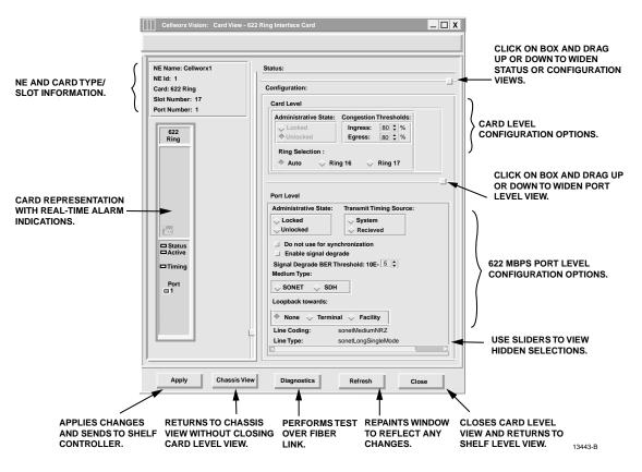
Figure 751-1. 622 RIC Shelf Level GUI Configuration Screen
